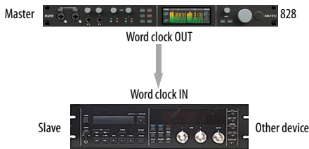
Figure 4-11: Slaving another digital audio device to the 828 via word clock. For the 828 clock source, choose Internal (or any source other than Word Clock , as daisy-chaining word clock is not recommended).
