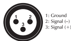
DMX-input XLR mounting-plug:
